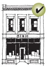
Mount a sign to fit within existing architectural features using the shape of the sign to help reinforce the horizontal lines of the building.
