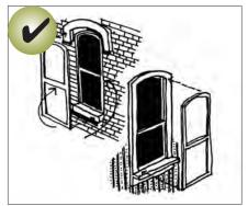
Appropriate: Install a storm window on the interior, when feasible. This will allow the character of the original window to be seen from the public way. If a storm window is to be installed on the exterior, match the sash design of the original windows.
